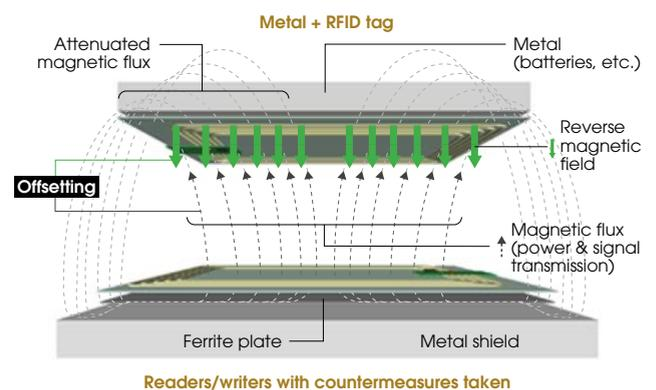
Using the ferrite plates applied in the readers/writers in mobile phones is difficult because of the thickness and physical strength. There's no space even for a shock-resistant resin ferrite. To install the 13.56MHz band RFID tags in mobile phones and to make them operate in a sufficient communication range, an eddy current reduction tool with magnetic flux convergence performance similar to that of the high-permeability ferrite plate in the Suica system readers/writers is required.
