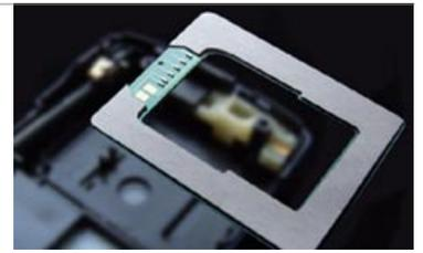
Also, the intense magnetic convergence effect (shield effect) caused by the industry's highest level high  $\mu'$  is the best countermeasure for battery packs which may affect the communication performance of mobile RFID systems.
