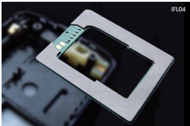
When a cheap 13.56MHz general-purpose RFID tag is used in terminals that are easily affected by the metal surfaces of devices such as mobile phones, a preset resonance frequency can be shifted to a higher frequency. Countermeasures to this problem must be taken.
