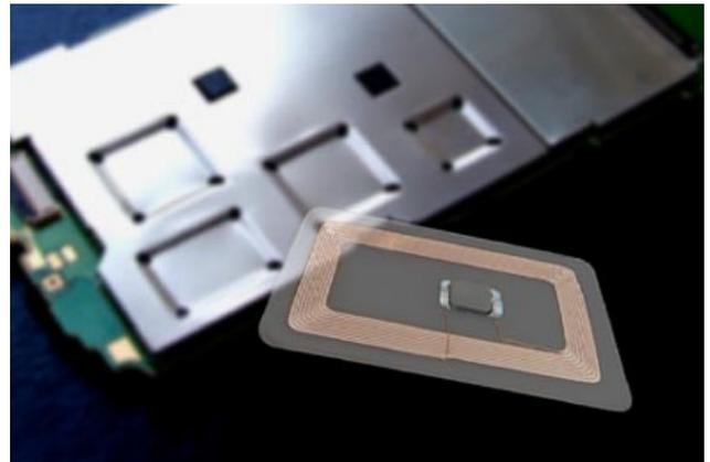
A similar problem also happens when a wireless tag is attached or closely positioned to the metal surface. In other words, the strength of the magnetic flux(the carrier wave of power and data) penetrating the inner periphery of the wireless tag antenna drastically attenuates due to the offsetting effect of the reverse magnetic field even when the card is held over the readers/writers with a sufficient magnetic field, causing a communication failure (as shown in the model diagram below).
