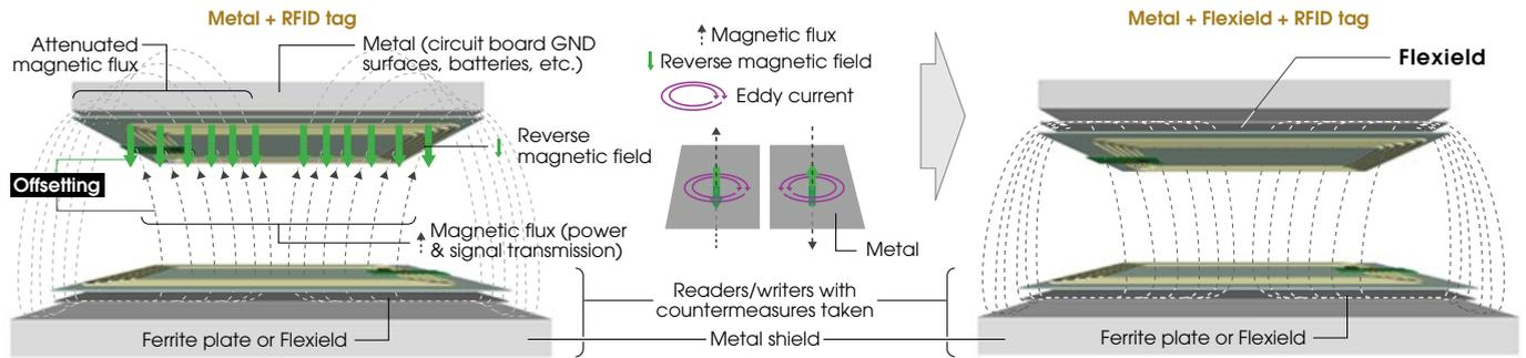
When the 13.56MHz carrier wave (magnetic field energy) penetrates the ground of a circuit board or metallized shield surface, eddy current will be induced on the metal surface, generating an unnecessary magnetic field that offsets the carrier wave.
