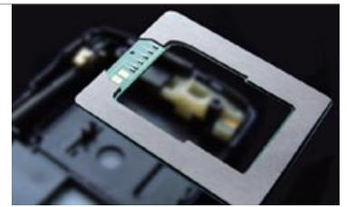
A sheet high-permeability material that's as thin and tough as the current wireless tags or even thinner and tougher — Developing such dedicated magnetic sheets and improving characteristics are essential for the further promotion and evolution of the 13.56MHz RFID system.
