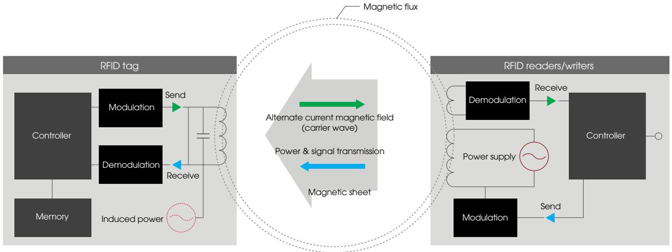
**The 13.56MHz RFID system operates in magnetic fields**
