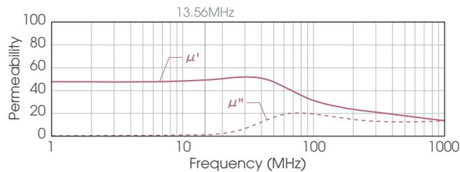
**IFL04** receives high regards as a low-loss/high Q type and can be attached directly to the built-in antennas of the 13.56MHz RFID systems. In addition to the **IFL04**'s thinnest specifications of 0.05mm and 0.1mm thick, a new material **IFL12**, which has the characteristics to deal with new demands, was developed.
